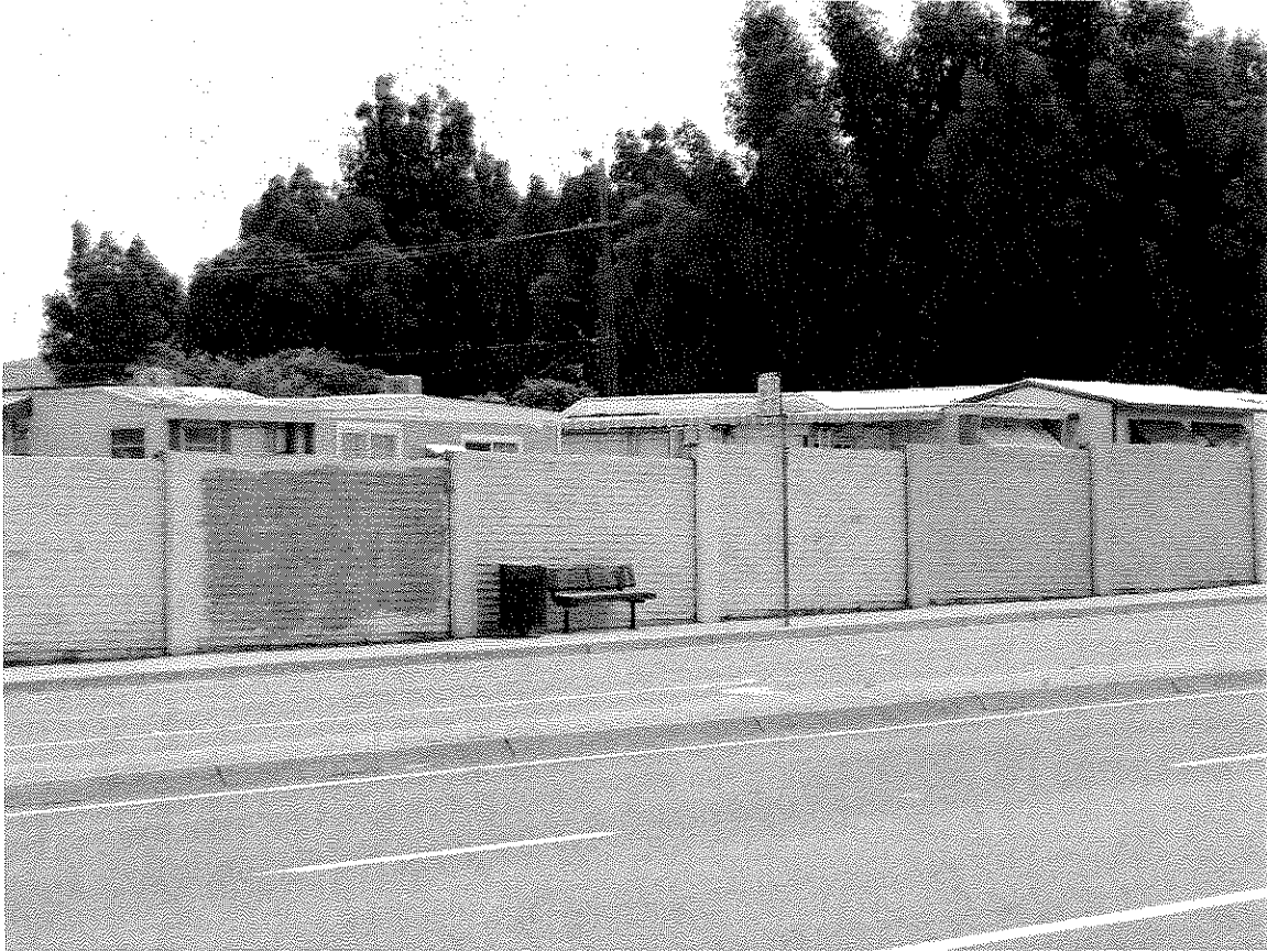
Photo 9. Tri Delta Transit bus stop on the east side of Bailey Road. The narrow sidewalk and presence of a soundwall provide little room for bus stop amenities such as a shelter. Three bus routes operate on this segment of Bailey Road.
